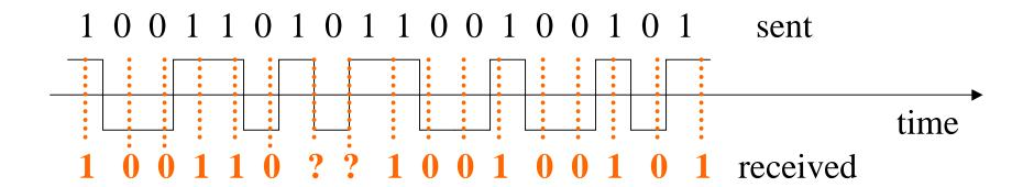
In wireless channels: multipath, shadowing, etc.
