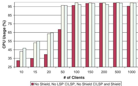
Figure 8: CPU Comparison for 100 Mbps Switch
