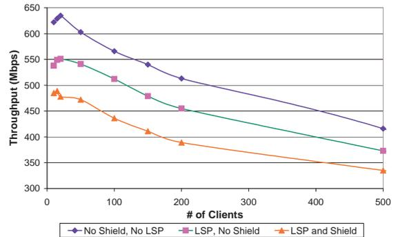
Figure 9: Throughput Comparison for 1 Gbps Switch
